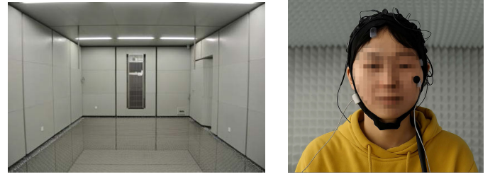
Fig. 2. Recording setup illustration. (a) Anechoic chamber used for dual-channel speech collection. (b) Participant wearing synchronized AC and BC microphones. EEG and EOG sensors were used for auxiliary multimodal acquisition. Facial features are blurred to preserve privacy.
