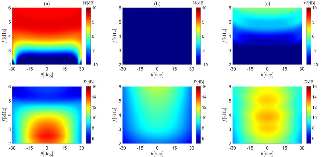
**Fig. 3.** WNG and DF as function of  $f$  and  $\theta$  for the competing methods: (a) ULA geometry, (b) dense geometry, and (c) proposed geometry.  $M = 6$ ,  $d_c = 0.5$  cm,  $A = 17.5$  cm,  $\theta_H = 30^\circ$ ,  $f_L = 2$  kHz,  $f_H = 6$  kHz, and  $\delta = -10$  dB.
