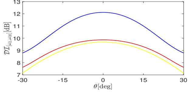
**Fig. 2.** Directivity index as function of  $\theta$  for the competing methods. The blue, red, and yellow lines mark the proposed, ULA, and dense geometries, respectively.  $M = 6$ ,  $d_c = 0.5$  cm,  $A = 17.5$  cm,  $\theta_H = 30^\circ$ ,  $f_L = 2$  kHz,  $f_H = 6$  kHz, and  $\delta = -10$  dB.
