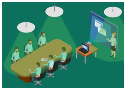
Figure 1. Conference room illustration with circular ceiling array covering multiple beamforming zones. Illustration courtesy of Stem Audio.
