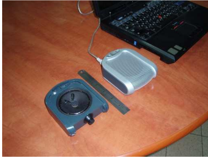
Figure 5.3: Experimental setup. A speakerphone (Phoenix Audio DUET Executive Conference Speakerphone) is connected to a laptop using its USB interface. Another speakerphone without its cover shows the placement of the built-in microphone and loudspeaker.
