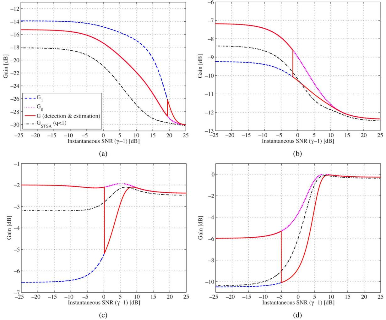
Fig. 2. Gain curves of  $G_1$  (dashed line),  $G_0$  (dotted line), and the total detection and estimation system gain curve (solid line), compared with the STSA gain under signal presence uncertainty (dashed-dotted line). The *a priori* SNRs are (a)  $\xi = -15$  dB, (b)  $\xi = -5$  dB, (c)  $\xi = 5$  dB, and (d)  $\xi = 15$  dB.
