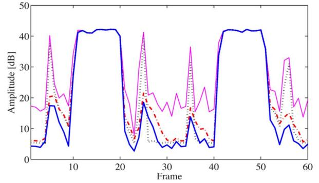
Fig. 6. Amplitudes of the STFT coefficients along time-trajectory corresponding to the frequency of the sinusoidal signal: noisy signal (light solid line), STSA with decision-directed estimation (dotted line), STSA with the modified *a priori* SNR estimator (dashed-dotted line), and simultaneous detection and estimation with the modified *a priori* SNR estimator (dark solid line).
