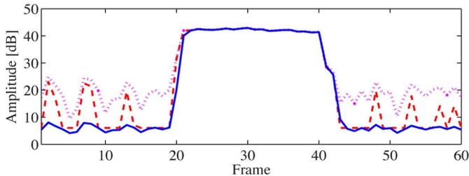
Fig. 4. Amplitudes of the STFT coefficients along the time-trajectory corresponding to the frequency of the sinusoidal signal: noisy signal (dotted line), spectral subtraction (dashed line), and simultaneous detection and estimation (solid line).
