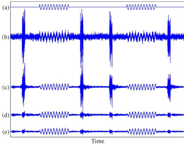
Fig. 5. Signals in the time domain. (a) Clean sinusoidal signal. (b) Noisy signal with both stationary and transient components. (c) Enhanced signal obtained by using the STSA and the decision-directed estimators. (d) Enhanced signal obtained by using the STSA and the modified *a priori* SNR estimators. (e) Enhanced signal obtained by using the detection and estimation approach and the modified *a priori* SNR estimator.
