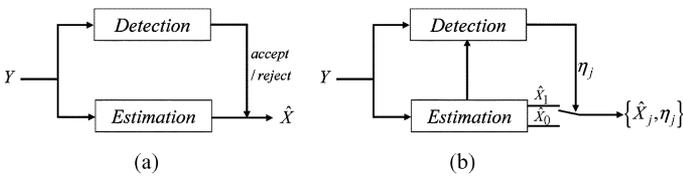
Fig. 1. (a) Independent detection and estimation system. (b) Strongly coupled detection and estimation system.
