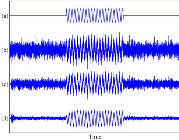
Fig. 3. Signals in the time domain. (a) Clean sinusoidal signal. (b) Noisy signal. (c) Enhanced signal obtained by using the spectral-subtraction estimator. (d) Enhanced signal obtained by using the detection and estimation approach.
