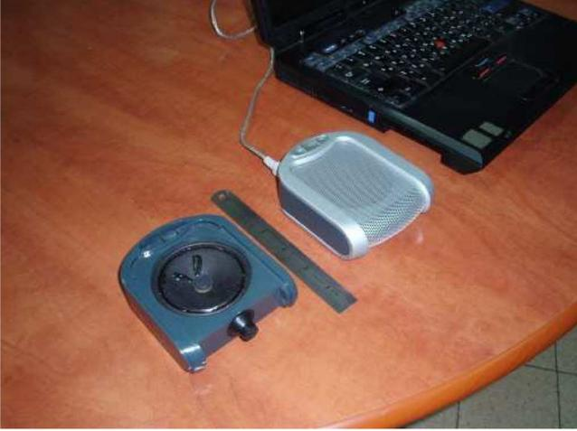
Fig. 4. Experimental setup. A speakerphone (Phoenix Audio DUET Executive Conference Speakerphone) is connected to a laptop using its USB interface. Another speakerphone without its cover shows the placement of the built-in microphone and loudspeaker.
