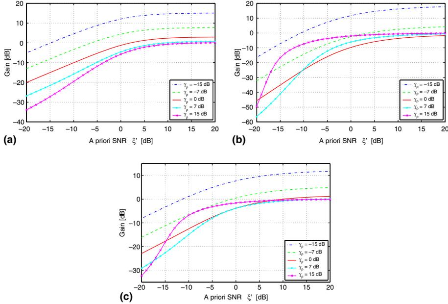
Fig. 2. Parametric gain curves describing the MMSE spectral power gain function  $H(\xi', \gamma_p)$  for different speech models: (a) Gain curves for Gaussian speech model, obtained by (18); (b) Gain curves for Gamma speech model, obtained by (19); (c) Gain curves for Laplacian speech model, obtained by (20).
