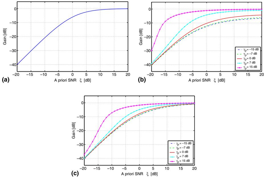
Fig. 1. Parametric gain curves describing the MMSE gain function  $G(\xi, \gamma_\rho)$  for different speech models: (a) Gain for Gaussian speech model, obtained by (9); (b) Gain curves for Gamma speech model, obtained by (10); (c) Gain curves for Laplacian speech model, obtained by (12).
