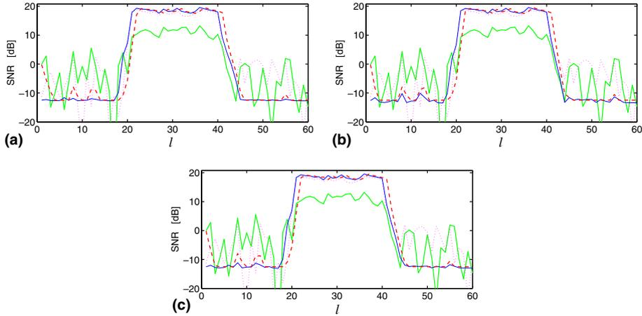
Fig. 3. SNRs in successive short-time frames for (a) Gaussian, (b) Gamma, and (c) Laplacian speech models: A posteriori SNRs  $\gamma_R$  (solid thin line) and  $\gamma_I$  (dotted line), decision-directed a priori SNR estimate  $\hat{\xi}^{DD}$  (dashed line), and noncausal a priori SNR estimate  $\hat{\xi}$  (solid heavy line).
