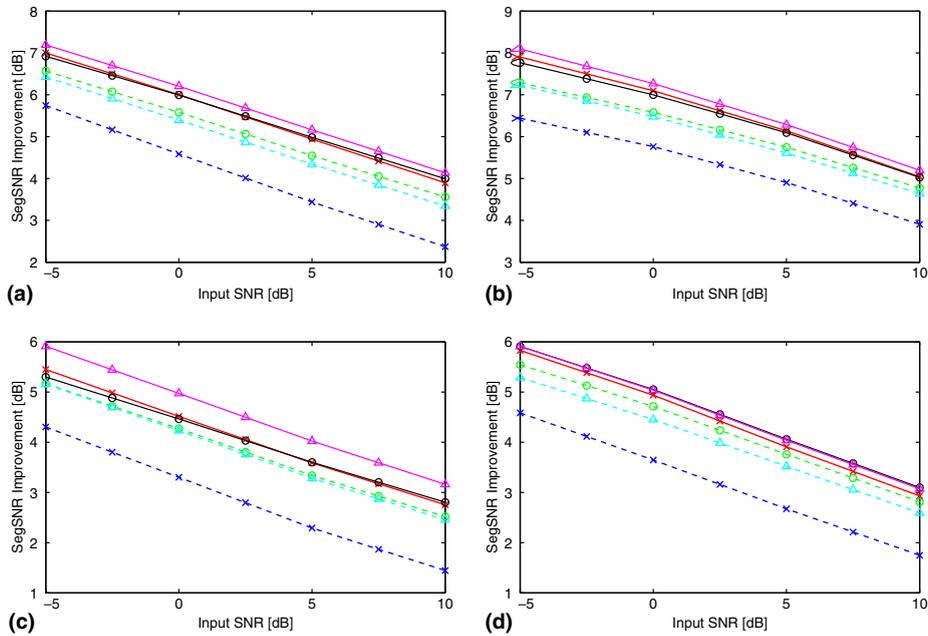
Fig. 4. Segmental SNR improvement for various noise types and levels, obtained by using Gaussian (×), Gamma (○) and Laplacian (△) speech models. The a priori SNR is obtained by either noncausal recursive estimation (solid lines) or by the decision-directed approach (dashed lines). (a) White Gaussian noise; (b) Car interior noise; (c) F16 cockpit noise; (d) Babble noise.
