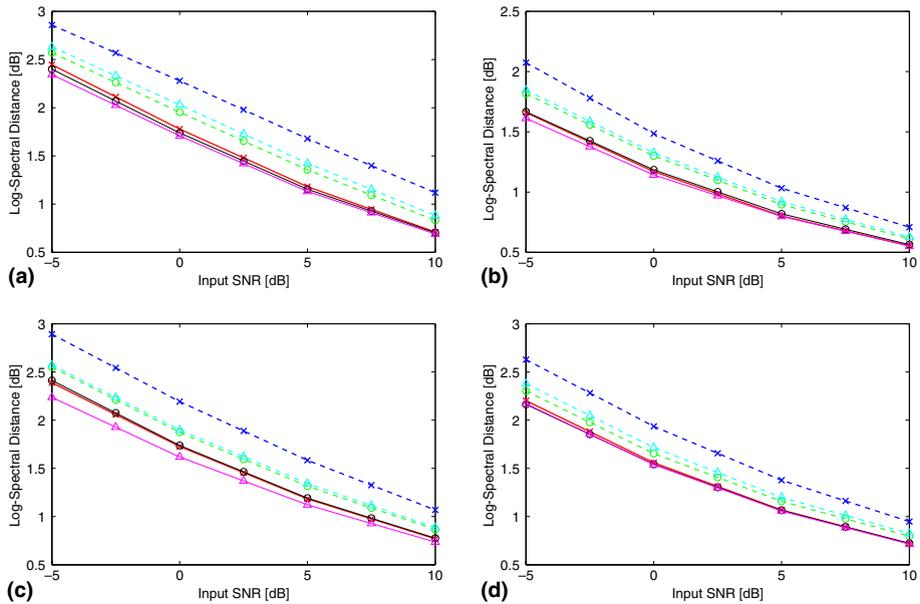
Fig. 5. Log-spectral distance for various noise types and levels, obtained by using Gaussian (×), Gamma (○) and Laplacian (△) speech models. The a priori SNR is obtained by either noncausal recursive estimation (solid lines) or by the decision-directed approach (dashed lines). (a) White Gaussian noise; (b) Car interior noise; (c) F16 cockpit noise; (d) Babble noise.
