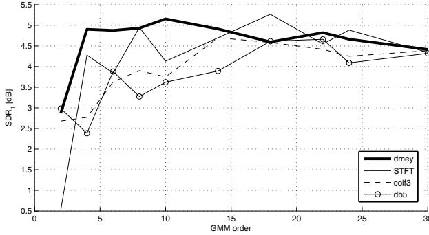
**Fig. 2.** Influence of the GMM model order on the signal to distortion ratio ( $SDR_1$ ) of the speech signal. STFT based algorithm [7] is compared to CSR-BS-WPD based algorithm.
