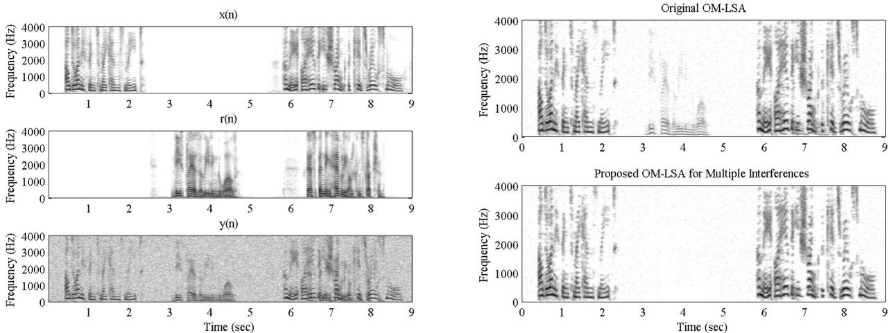
Figure 1: Spectrograms of the desired signal  $x(n)$ , the non-stationary interference  $r(n)$ , the microphone signal  $y(n)$ , and the original and modified OM-LSA using the non-causal *a priori* SNR estimator.
