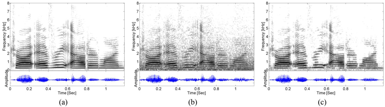
Figure 1: Speech spectrograms and waveforms. (a) Clean signal: "Try any other line."; (b) speech corrupted by factory noise with 5 dB SNR (LSD= 6.68 dB, SegSNR= 0.05 dB); (c) speech reconstructed by using 4-state model (LSD= 3.14 dB, SegSNR= 6.76 dB).
